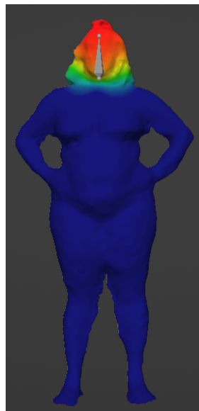
Figure 2.5: "Head" armature-controlled parts (the degree of redness indicates the degree of influence of the corresponding armature)
